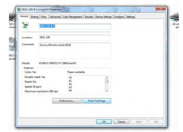
You can also **print a test page** from the printer list by going to printer properties.
